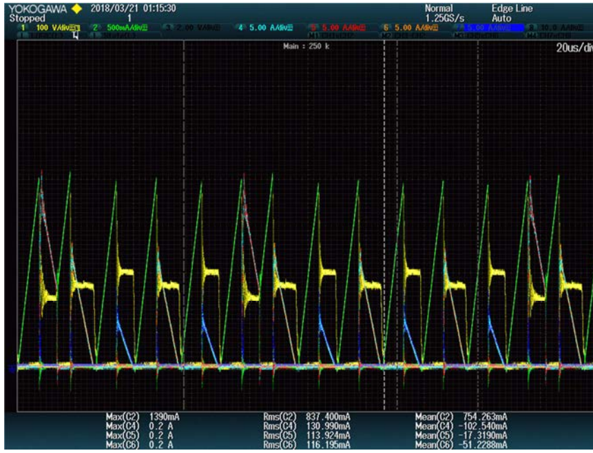
Figure 35 – Zoom on Transformer Pri/Sec Current Waveform.
