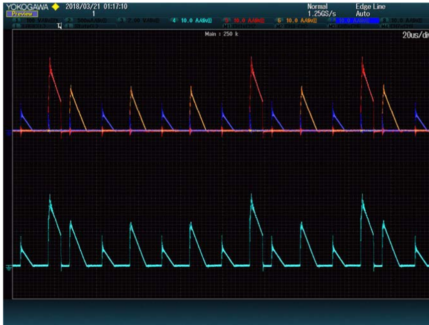
Figure 36 – Zoom on Transformer Sec Current Waveform.
