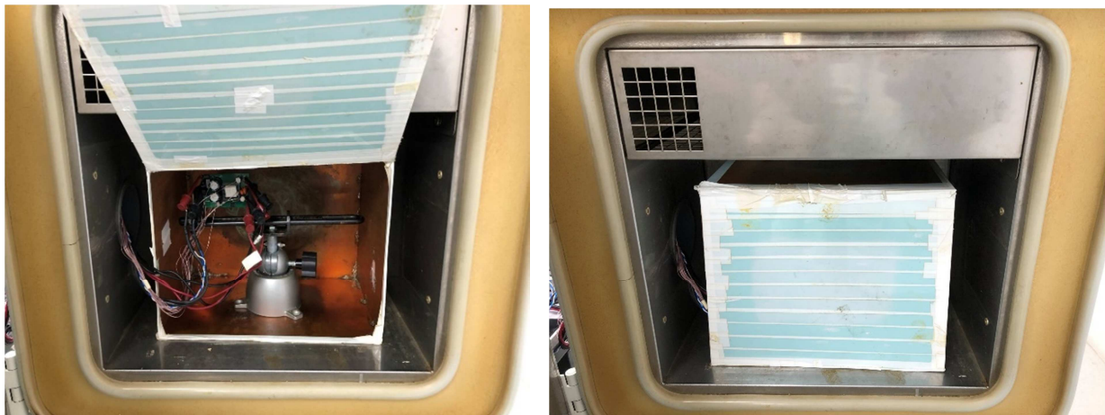
Figure 88 – Thermal Performance Set-up Using Thermal Chamber.
