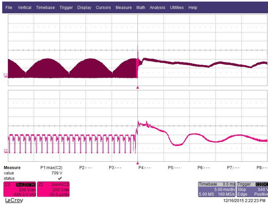
Figure 135 – (+)3 kV Differential Surge, 90° Phase.
