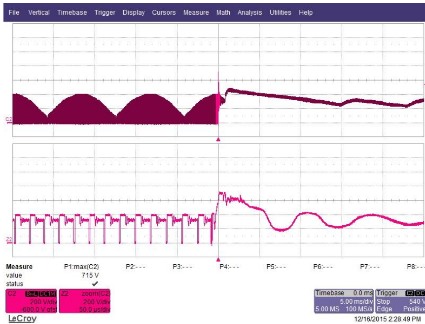
Figure 139 – (-)3 kV Differential Surge, 270° Phase. Upper: V_{DRAIN} , 200 V / div., 5 ms / div. Lower: V_{DRAINzoomed} , 200 V / div., 50 \mu s / div. Peak V_{DRAIN} : 715 V.
