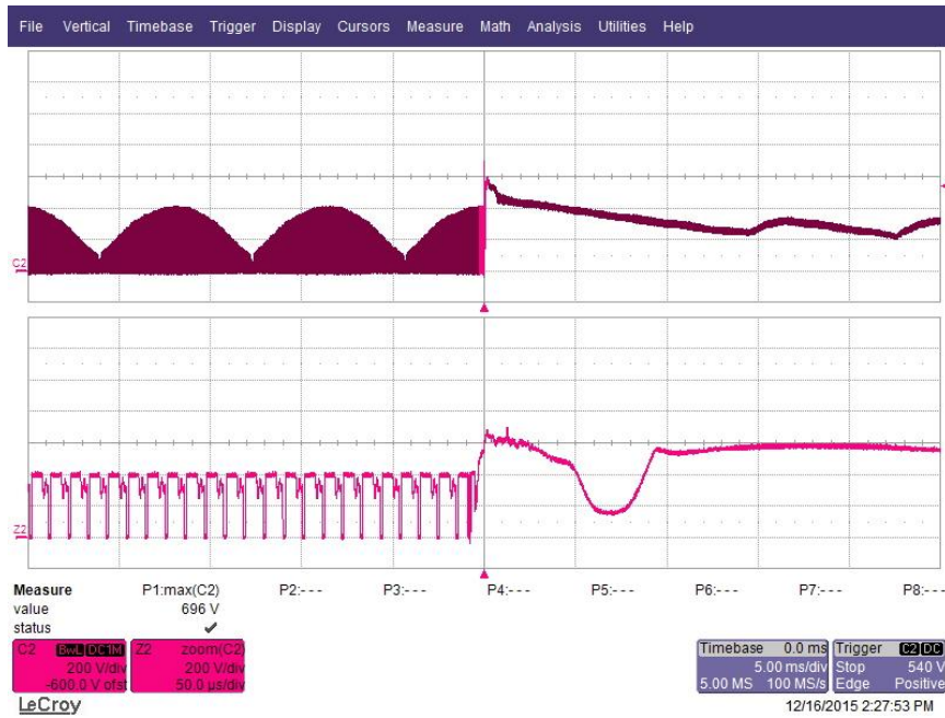
Figure 138 – (-)3 kV Differential Surge, 90° Phase. Upper: V_{DRAIN} , 200 V / div., 5 ms / div. Lower: V_{DRAIN\text{zoomed}} , 200 V / div., 50 \mu s / div. Peak V_{DRAIN} : 696 V.
