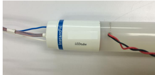
Figure 20 – Set-up, the power supply fitted inside T8 tube for actual application measurement.
