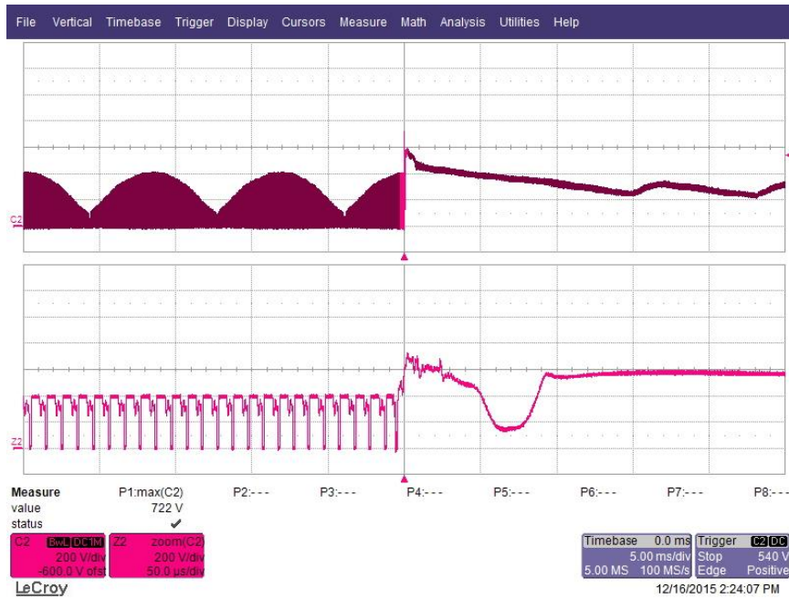
Figure 136 – (+)3 kV Differential Surge, 270° Phase. Upper: V_{DRAIN} , 200 V / div., 5 ms / div. Lower: V_{DRAIN} zoomed, 200 V / div., 50 \mu s / div. Peak V_{DRAIN} : 722 V.
