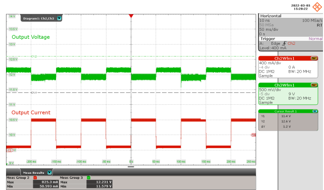
Figure 94 – Transient Output Waveforms. 265 VAC. Output Current: 400 mA / div., 50 ms / div. Output Voltage: 500 mV / div., 50 ms / div.. Load Transient: 10 % - 100%. Duty Cycle, Slew Rate: 50%, 0.8 A / \mu s. Frequency: 10 Hz. V_{MAX} : 12.231 V, V_{MIN} : 11.579 V.
