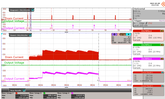
Figure 34 – Drain Current and Output Waveforms. 85 VAC Input. Drain Current: 2 A / div., 1 s / div. Output Voltage: 6 V / div., 1 s / div. Output Current: 2 A / div., 1 s / div. Zoom = 10 ms / div.
